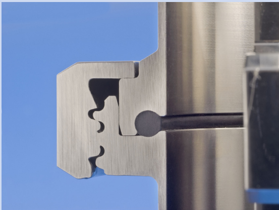
CROSS-SECTION GASKET AREA DIN 11853 COUPLING
